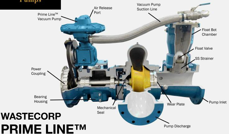
Wastecorp Prime Line™ technology is capable of rapid (50 CFM) self-priming up to 28 Feet (8 meter) depths below the pump. The fast priming positive displacement vacuum pump ensures that no water carry-over occurs thanks to the reliable inlet float box chamber.
