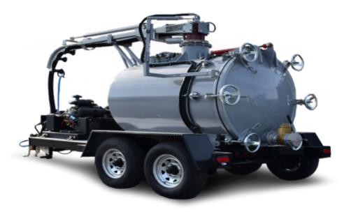
SUPER DUTY® HYDROVAC TRAILERS Designed and Manufactured by Wastecorp Pumps in USA and/or Canada.
