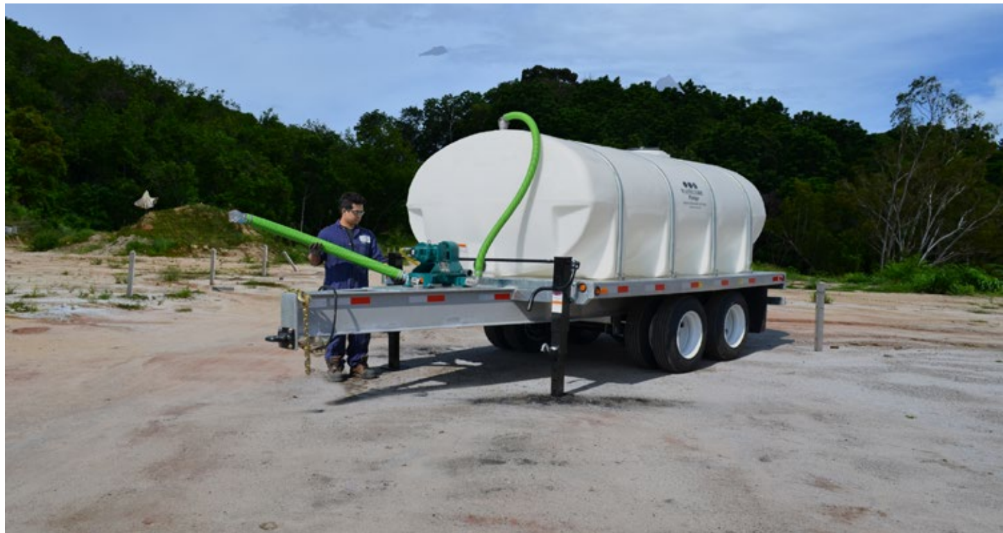
HW-2000 Series. 2035 gallon tank, dually trailer, dual jack, galvanized deck and frame. Mud Sucker mechanical AOD pump motor technology. Installation used on a US Army base for pumping out septic systems at remote training facility.
