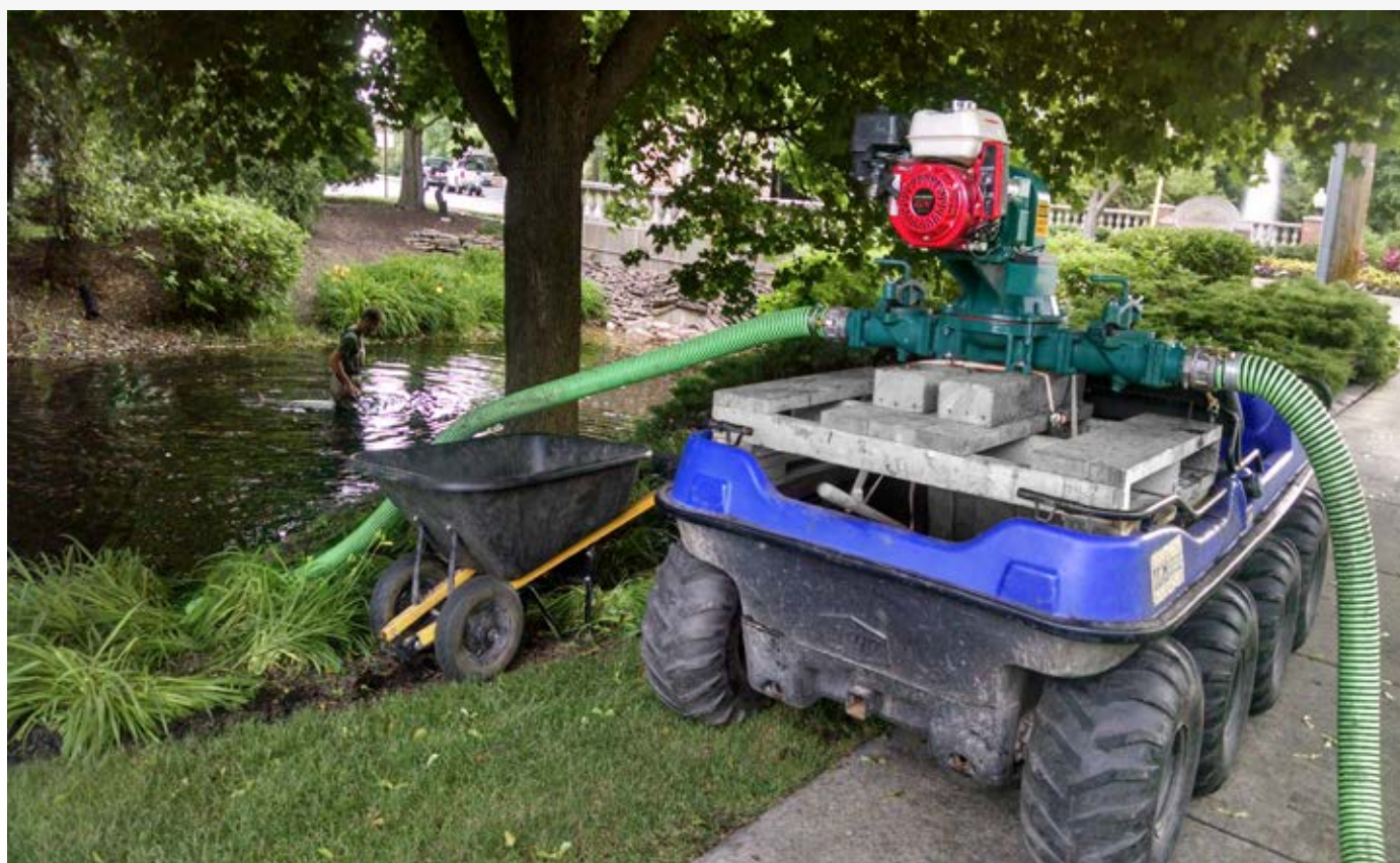
Mud Sucker 3FAC-M (stationary model) being used for a lagoon dredging operation. Pump transfers up to 80 GPM of wastewater and solids. Shown with an e-start Honda engine. Wheel kits, accessories and alternate configurations available.
