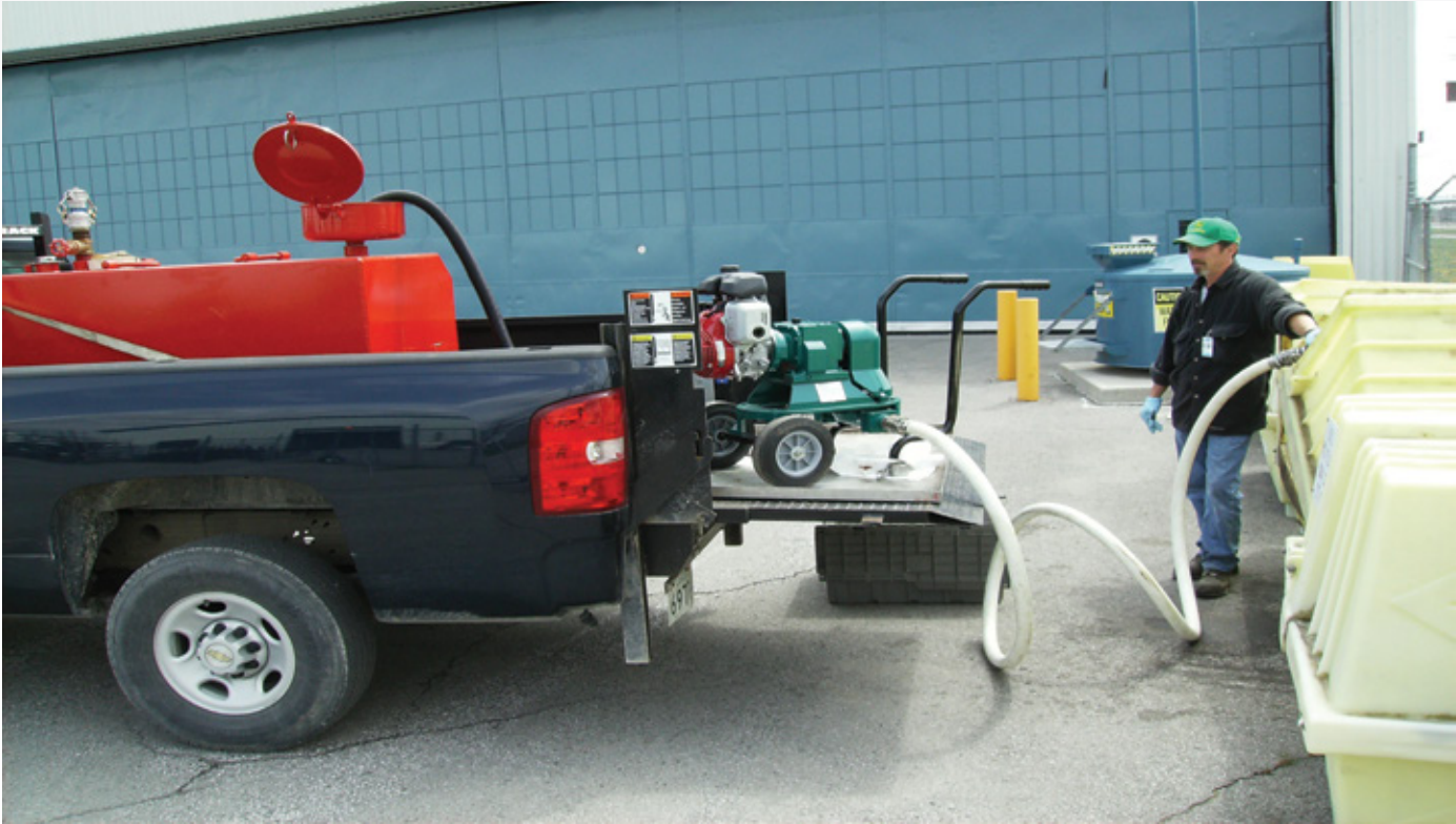
Mud Sucker 2FAC-M with a 3 hp Honda engine. Shown on a military base pumping waste oil. Non-collapsible suction and discharge hoses are available.
