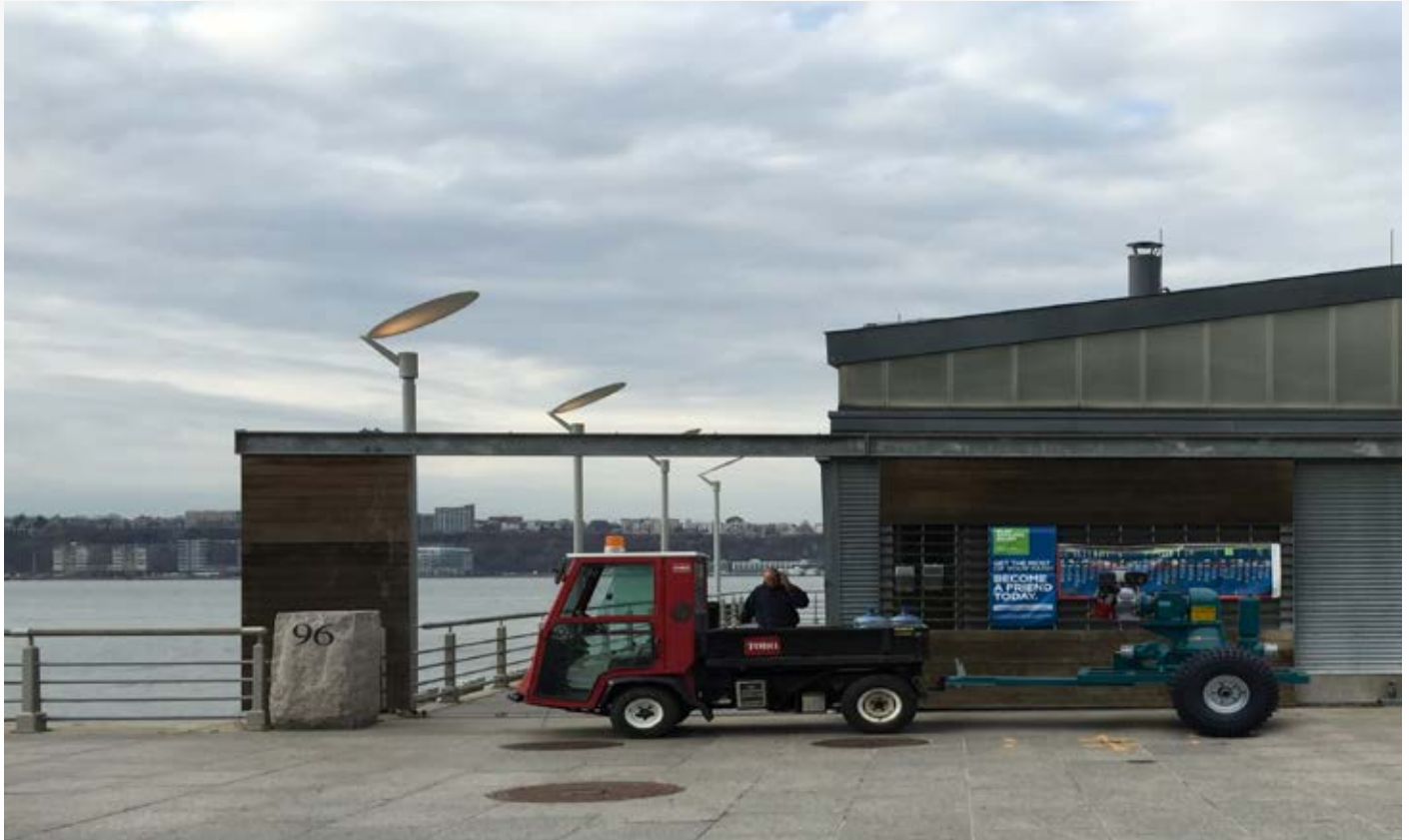
The Mud Sucker 3BM-T conquers debris laden waste at sewer reconstruction projects, mining and many construction related applications. Shown: Mud Sucker 3BM-T off road trailer model with turf tires to reduce impact on existing landscaping.
