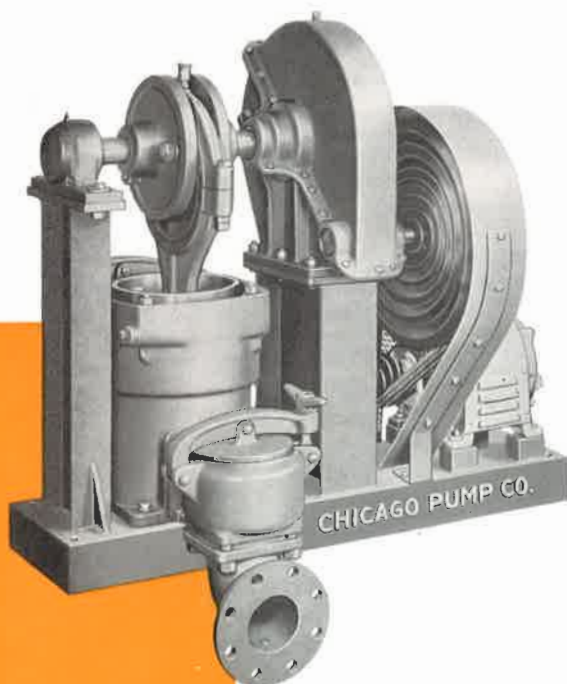
Fig. 2841—"Chicago" Single Plunger Sludge Pump with V-belt drive. Air chamber furnished similar to that in Fig. 2843, but without manifold.
