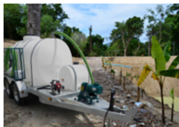
Waste + Water Tanks With Separate Pumps
