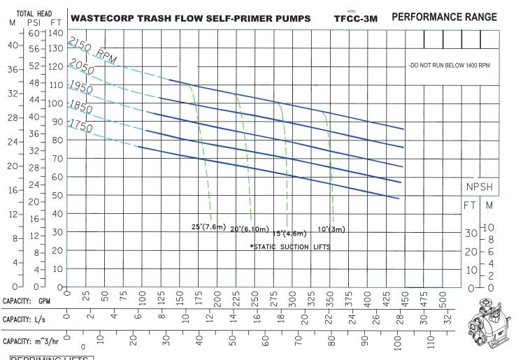
REPRIMING LIFTS PUMP SPEED 1450 RPM 1550 RPM 1650 RPM 1750 RPM 1850 RPM 1950 RPM PUMP SPEED 2050 RPM 2150 RPM 20 Ft. 21 Ft. 22 Ft. 22 Ft. 25 Ft. 25 Ft. GPM x FT x SG M<sup>3</sup>/HR x M x SG 367 x Efficiency KW= -3960 x Efficiency
