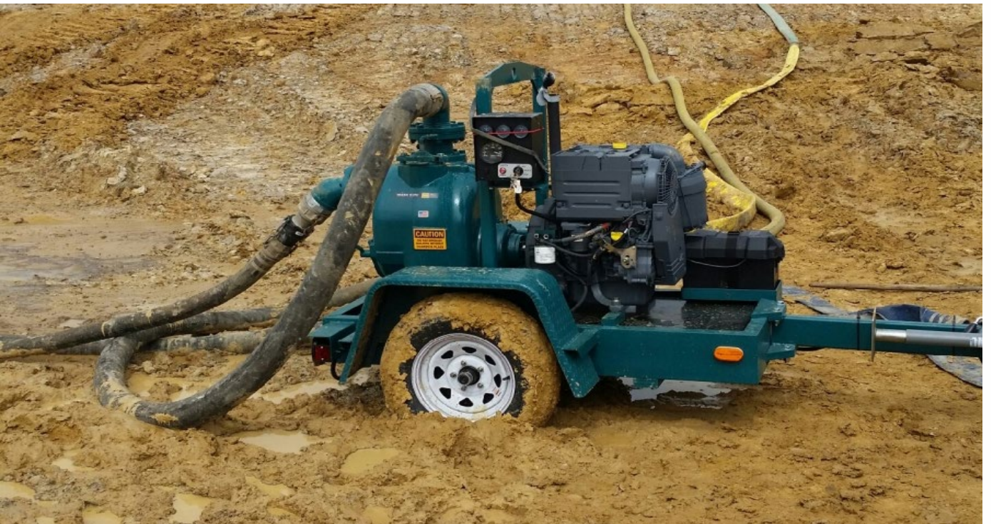
TRAILER MOUNTED TRASH PUMPS Shown TFCC-6ML pumping slurry from an industrial lagoon. Deutz diesel engine, DOT approved lighting package and electronic start enhance pumping outdoors.
