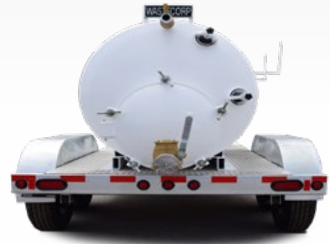
TVP-1000, 1000 gallon model shown with galvanized frame, diamond plate deck and DOT compliant trailer system. Optional extended deck model shown.
