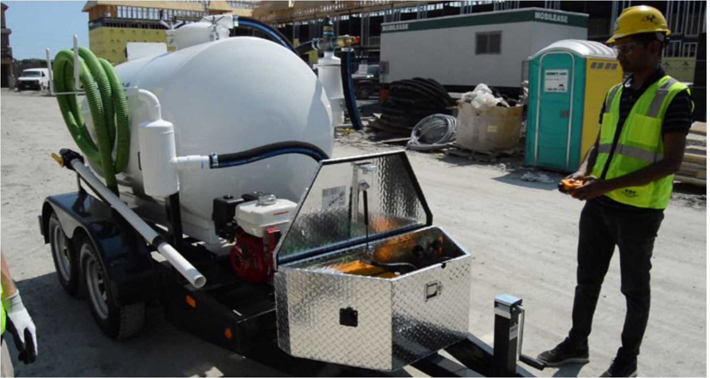
Super Duty TVP-600 Series vacuum pump, trailer mounted with Tilt-N-Go, tilt tank feature. Operator controls tilt function with remote control. wireless functions also available. Used to pump out portable toilets on construction sites.
