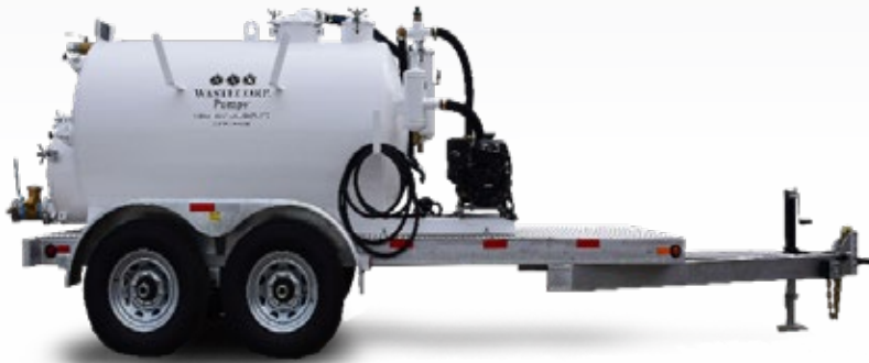
TVP-1000, 1000 gallon model shown with galvanized frame, diamond plate deck and DOT compliant trailer system. Optional extended deck model shown.
