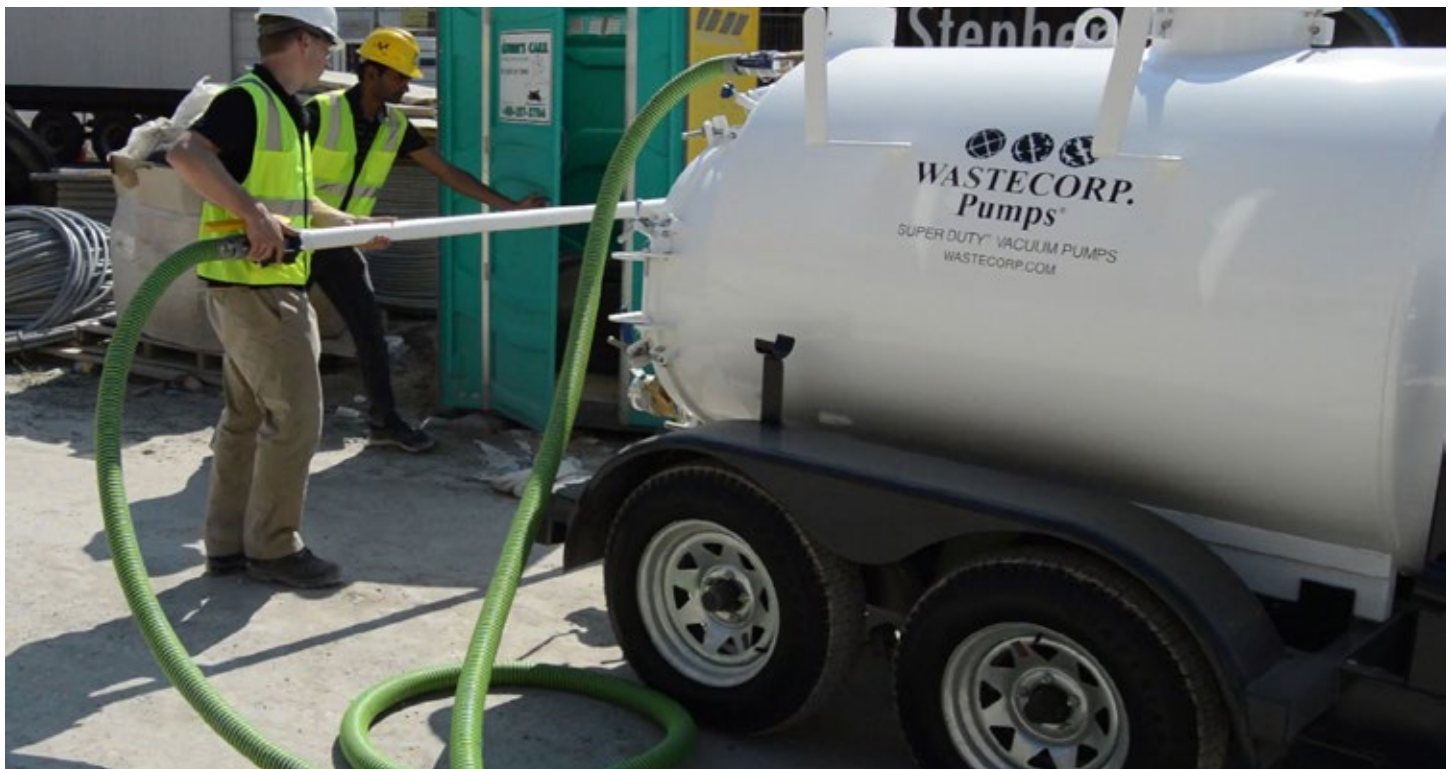
Super Duty TVP 450-200, dual compartment mounted vacuum pump. 450 gallon waste, 200 gallon fresh water compartment. Used on a construction site to pump out portable toilets and refill with fresh water. Also includes a high pressure water pump to rinse down area.
