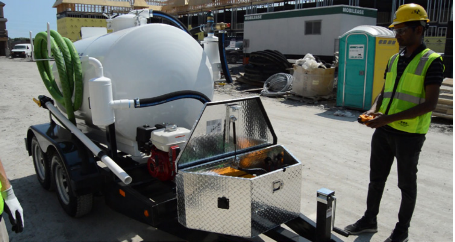
Super Duty TVP-600 Series vacuum pump, trailer mounted with Tilt-N-Go, tilt tank feature. Operator controls tilt tank function with remote control. wireless functions also available. Used to pump out portable toilets on construction sites.
