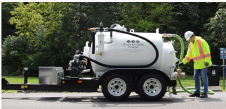
TVP-450, 450 gallon model shown with DOT compliant trailer and optional storage bin.
