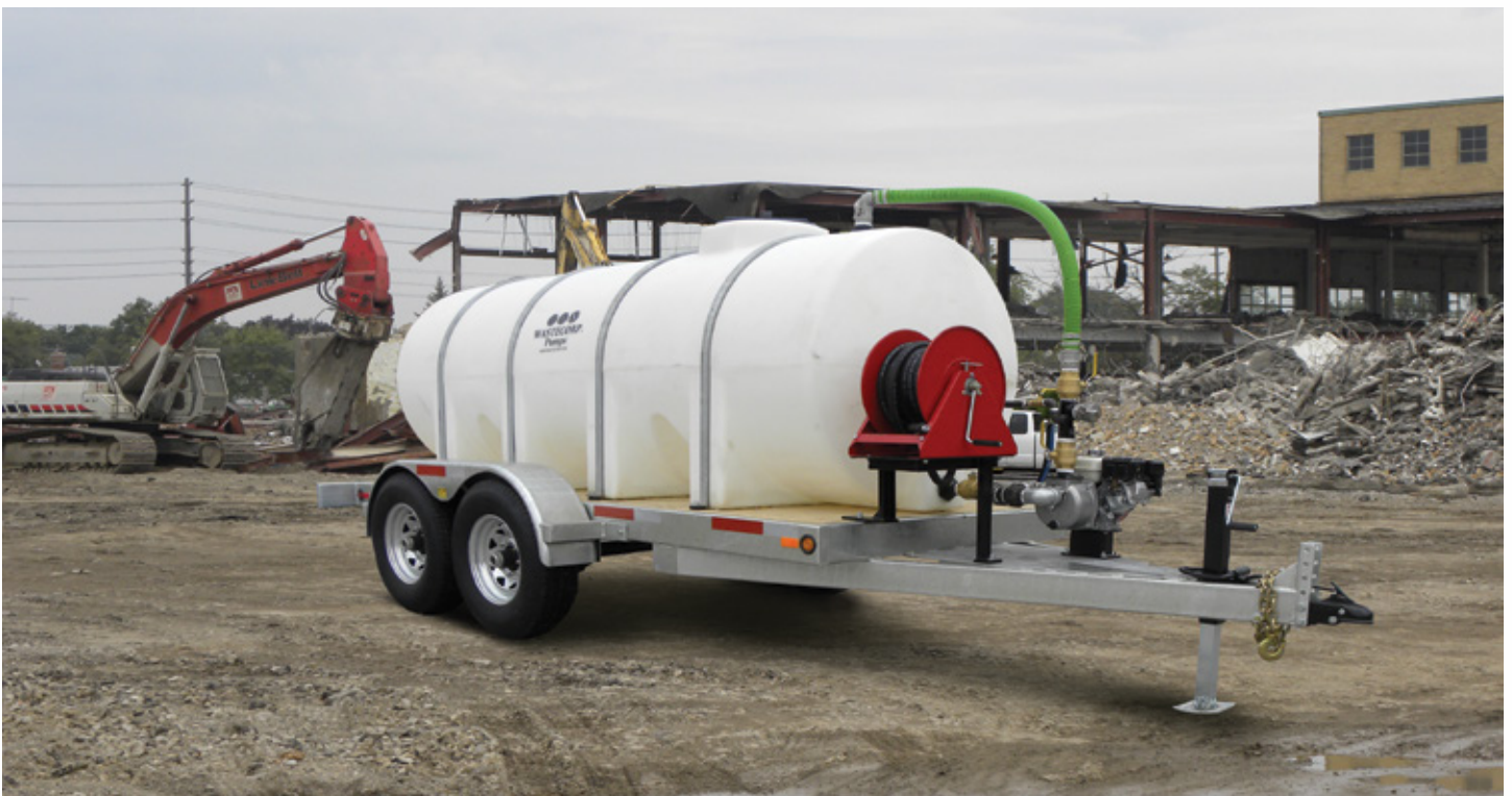
WATER TRAILERS DESIGNED FOR LONG LIFE IN PUNISHING CONDITIONS Shown: THE WT-1000 Series with a 1025 gallon tank and tandem axle galvanized trailer on a public utilities site. Custom hose reel part no. 62664-00 selected with rear sprayers.
